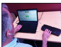
Figure 6: visually impaired user listening & using the Liblouis Braille system simultaneously.
